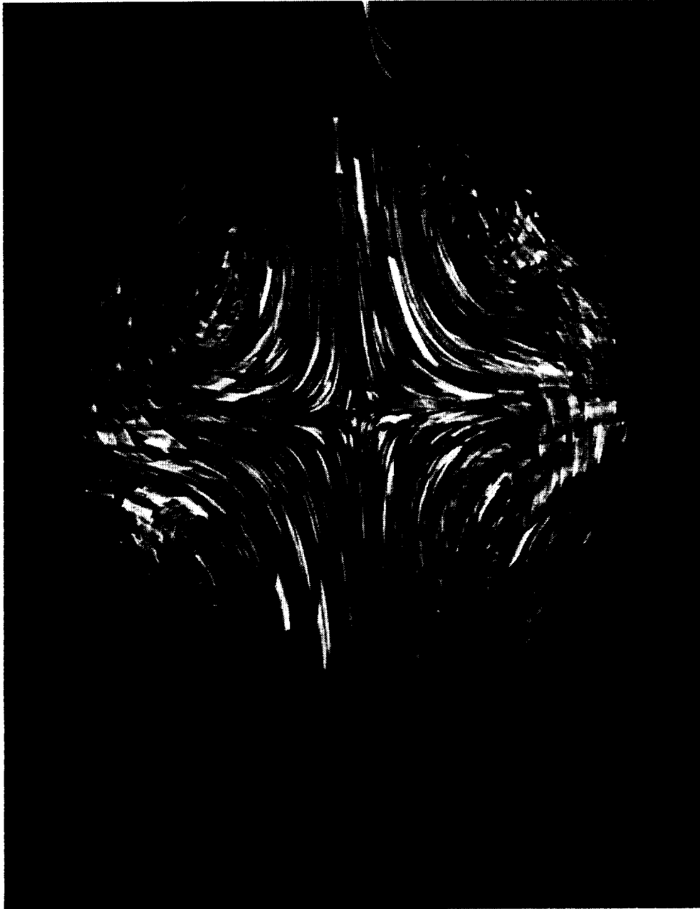
Figure 3 Tracer particles-based visualization of the internal flow of a freely suspended drop undergoing large amplitude drop shape oscillations. Steady convective flows have been observed in addition to the oscillatory motion. Data from E. Trinh and T. Wang, J. Fluid Mech. 122 , 315 (1982)
