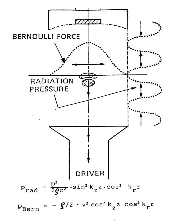
Fig. 2: Drop levitation in an one-axial acoustic levitator (schematical)
