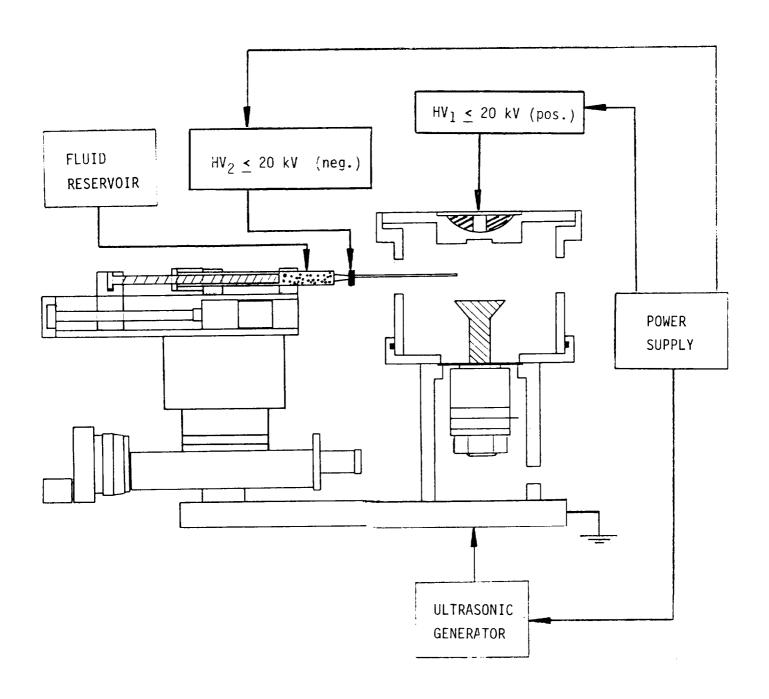
Fig. 7: Block diagram of the Electrostatic-Acoustic-Hybrid Levitator
