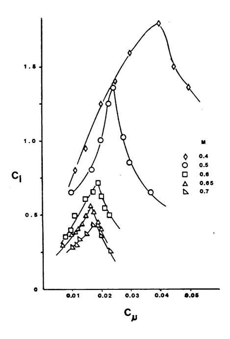
Figure 7.- Plot of lift coefficient with blowing at a range of freestream Mach numbers.
