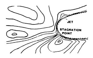
was to increase the effective camber of the airfoil, and hence, the circulation. Flow on the lower surface of the airfoil was relatively uniform as indicated by the few broad fringes there. The wake was deflected downward by the circulation and spread rapidly as a result of the vertical momentum introduced by the jet.
