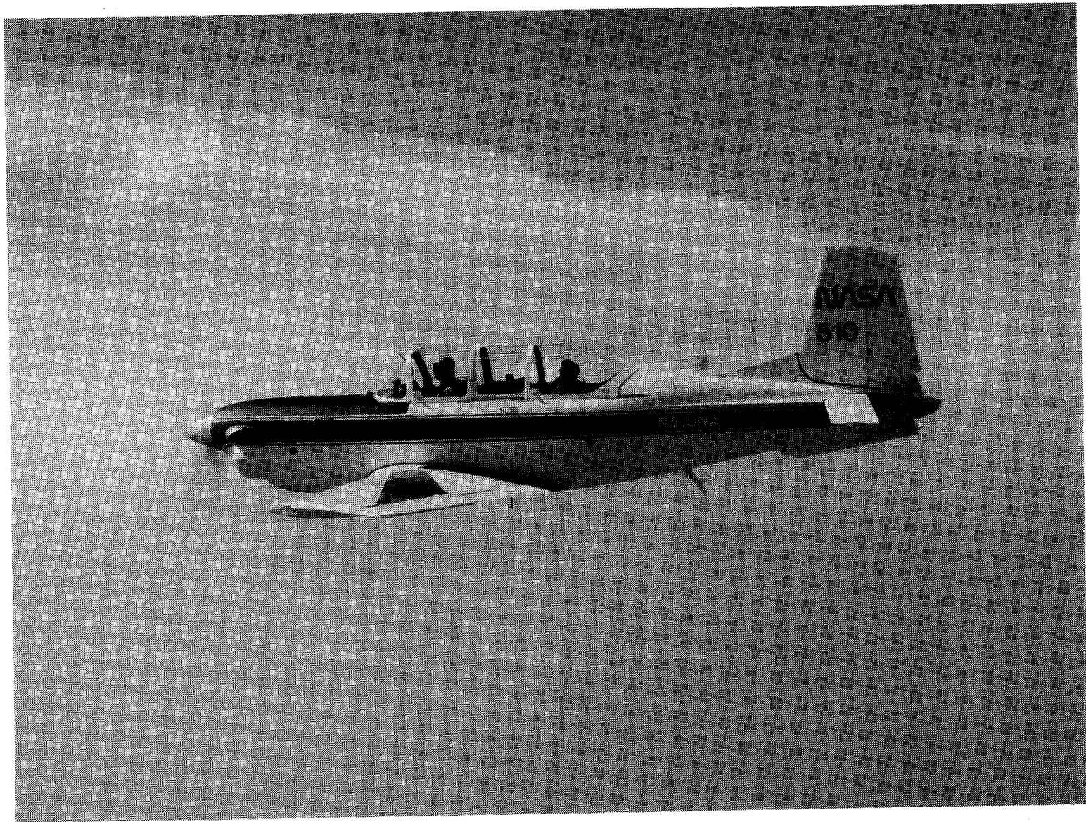
Figure 2. Observation Aircraft. Beech T-34C equipped with wingtip-mounted video cameras to determine separation distance.
