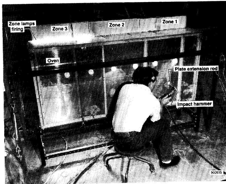
Figure 4. Enclosed oven used to heat an aluminum plate.
