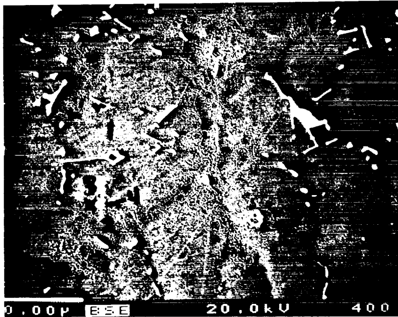
Figure A. Photomicrograph of a MAR-M 246 + Hf sample directionally solidified at 1 cm/min without a magnetic field. Sample 009AbMMO. Photo was taken from the upper portion of the sample (i.e., last to solidify). Backscattered electron image.
