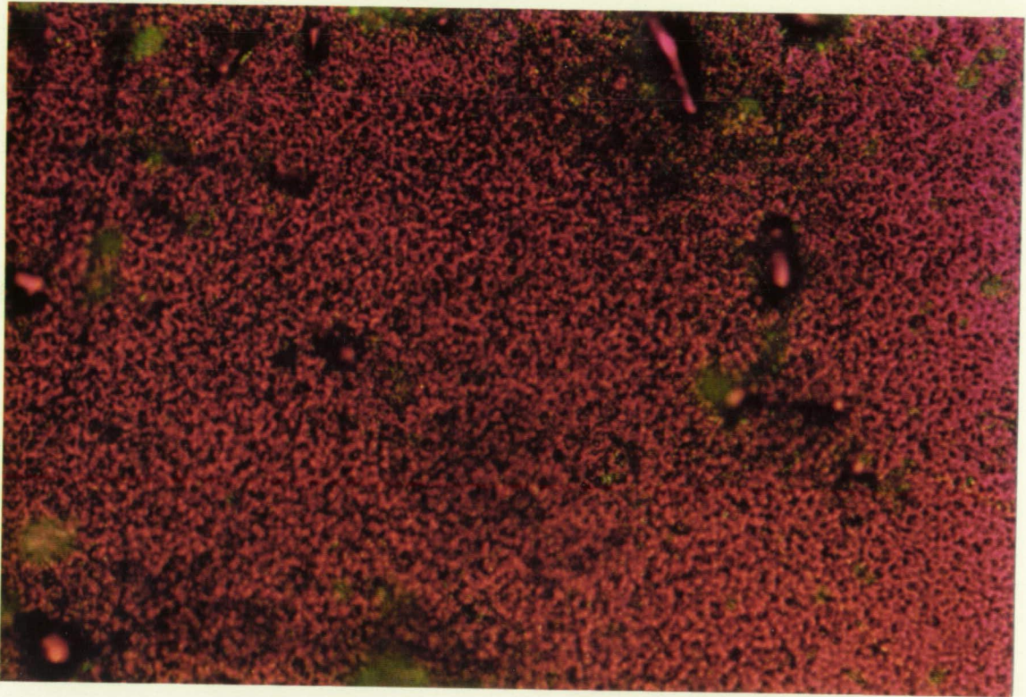
Fig.5 Photomicrograph of Ni-based superalloy MAR-M246(Hf) before heat treatment (Sample # 203H) using first order red compensator at 666x
