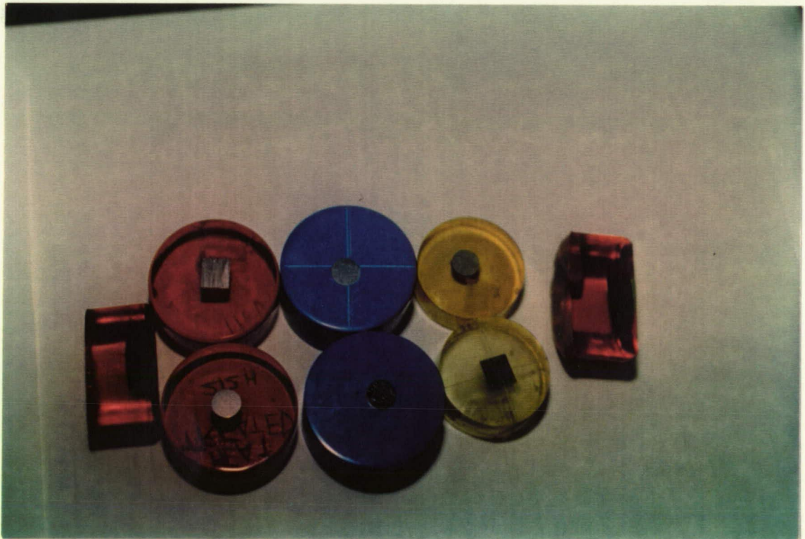
Fig.2 Ni-based superalloy MAR-M246(Hf) in the hot and cold molds
