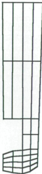
Figure 14.—Predicted shape of the smallest repeating segment after 200 cycles (data from ref. 3).
