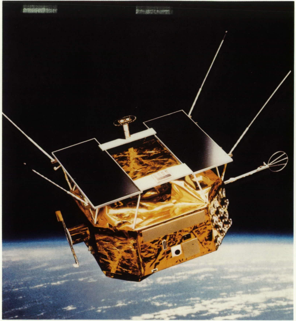
Typical flight configuration of CRRES showing booms extended and magnetic field loop antenna. (Note canister ejection ports at right).
