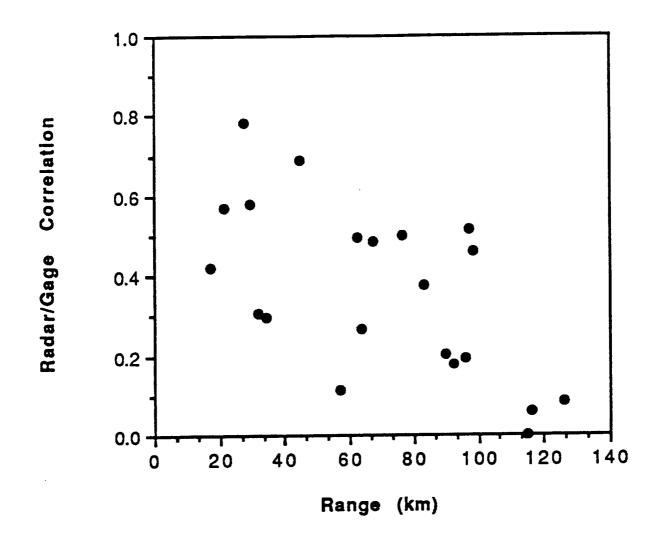
Figure 7. Radar-raingage correlation of hourly data for the co-located points.
