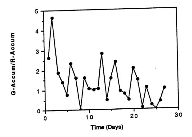
Figure 6. Time series of daily bias of the radar-rainfall. The bias is defined as the ratio of gage to been mean areal values.
