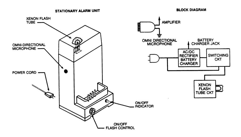
FIGURE 4 STATIONARY ALARM UNIT
