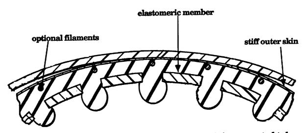
Applied force is damped as elastomer flows throgh inner nested tube
