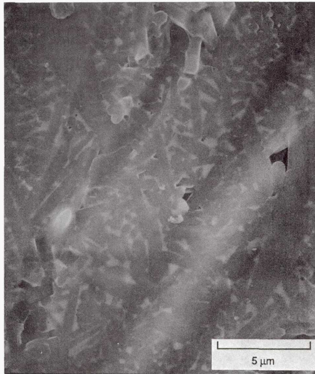
Figure 4.—Glassy region connected to a large grain that induced strength failure.
