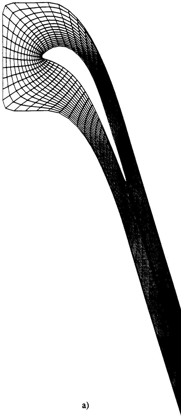
Figure 7.24. 73x17 Computational Mesh for Inviscid Turbine Calculations. (a) Global View (b) Leading Edge Detail (c) Trailing Edge Detail
