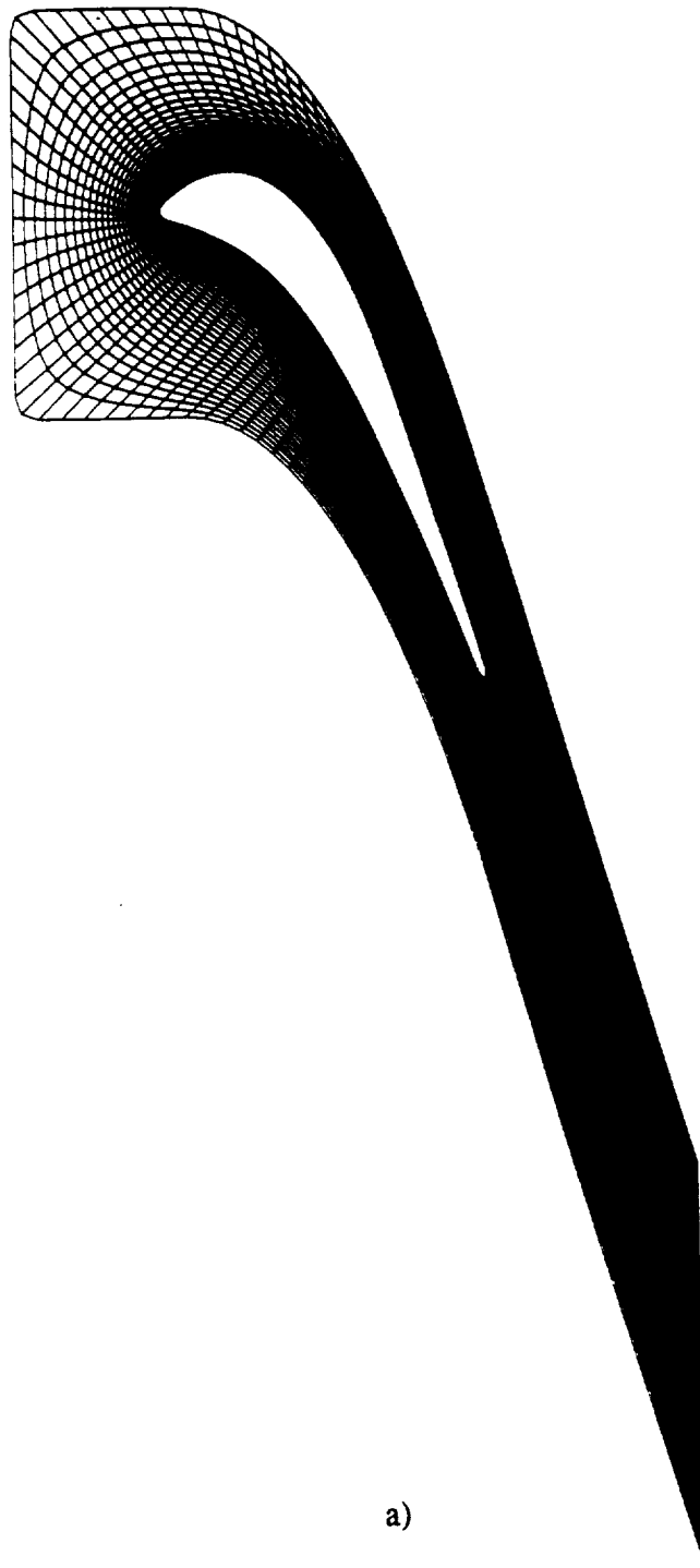
Figure 7.27. 129x41 Computational Mesh for Viscous Turbine Calculations. (a) Global View (b) Leading Edge Detail (c) Trailing Edge Detail
