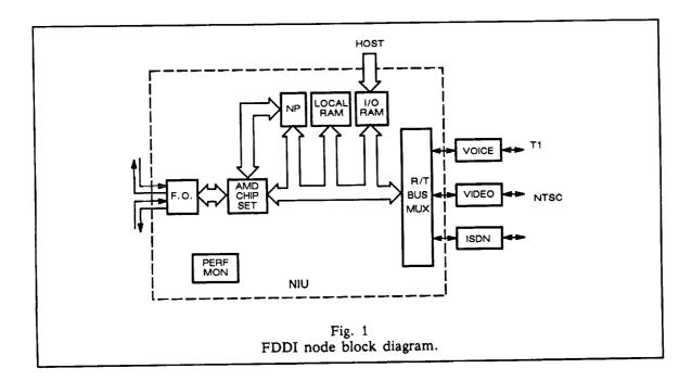
using the 16-bit Node Data and Node Address busses. The SUPERNET chip-set and the buffer memory make their status available to the NP, which has complete control over them.
