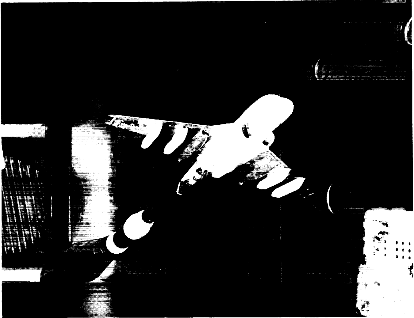
Figure 30. EA-6B model mounted in NTF.
