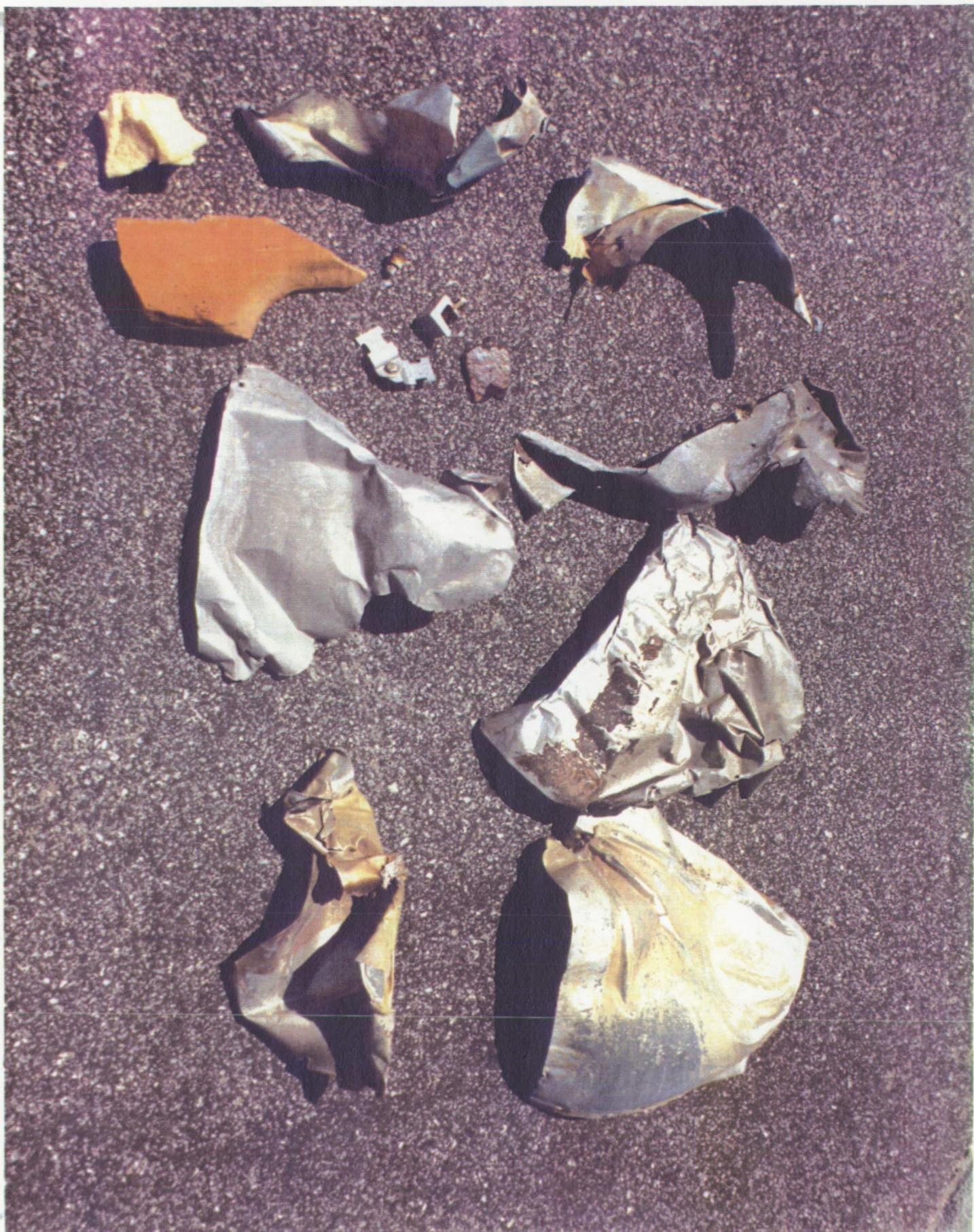
Post launch debris included pieces of thin sheet metal from a chilled water pipe on the FSS/RSS 107 foot level crossover. No flight hardware was found.
