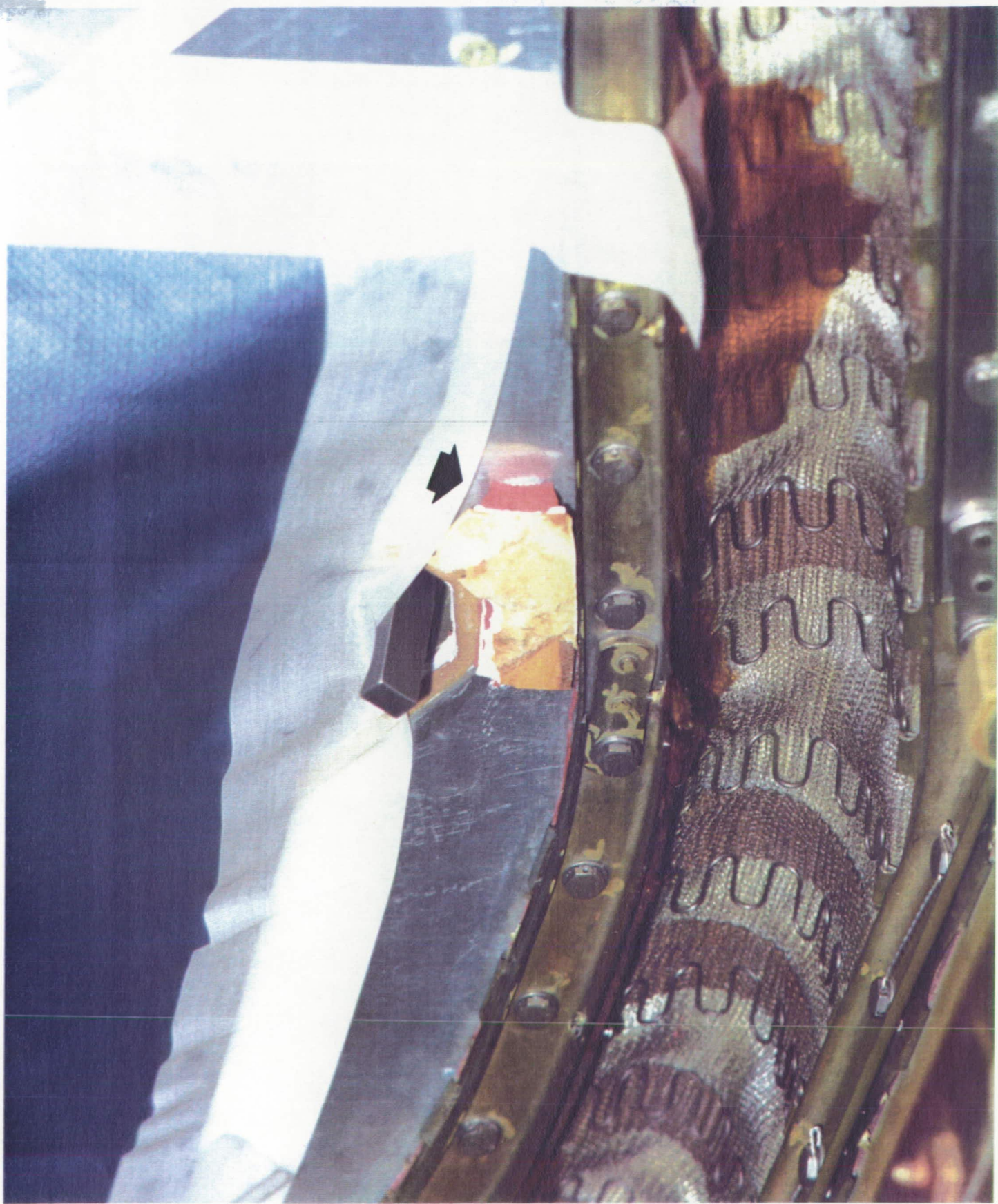
2-inch piece of umbilical purge seal, which should have remained attached to the External Tank, adhered to the Orbiter side of the LH2 ET/ORB umbilical plate
