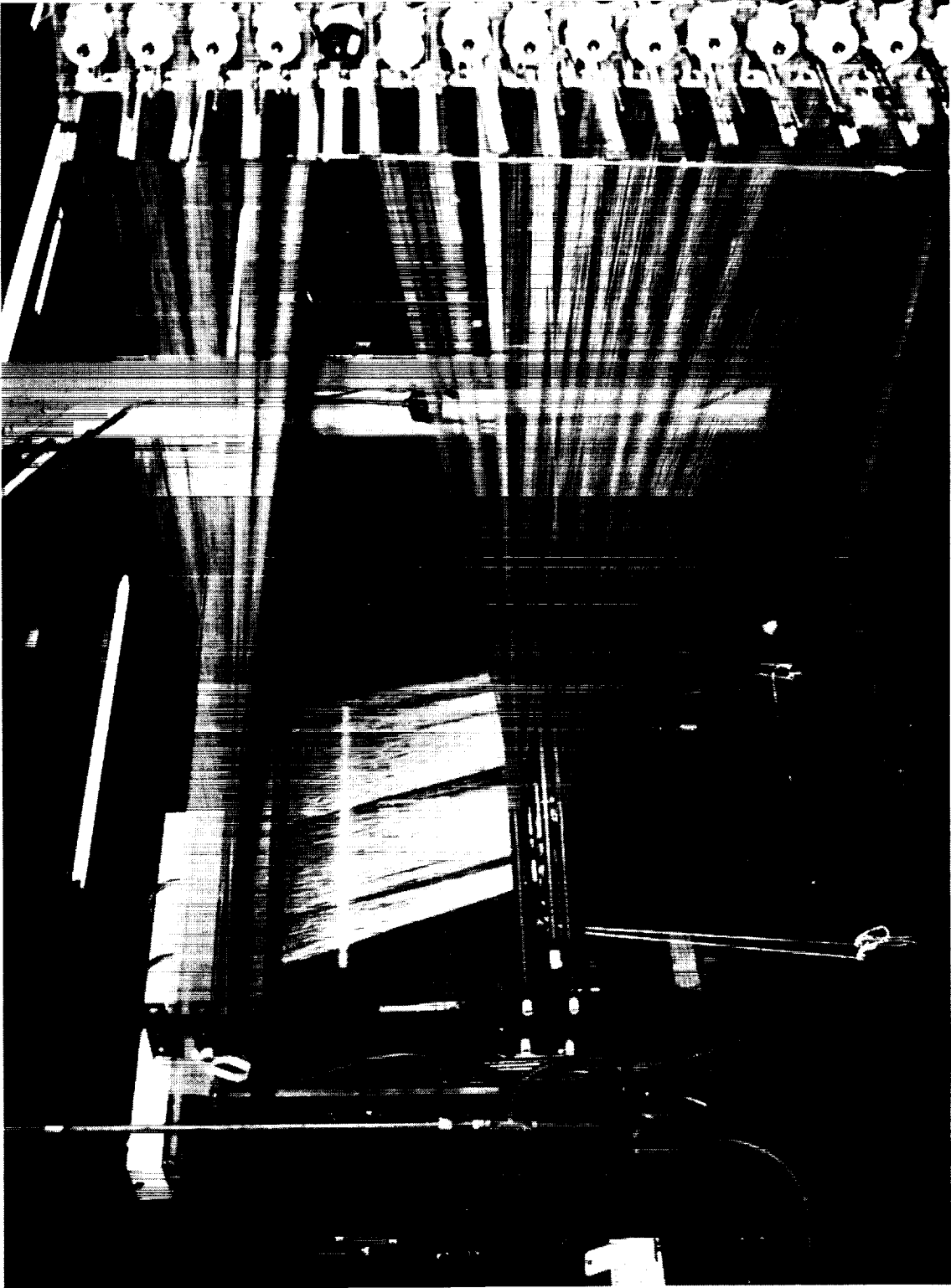
Figure 3-3 NEXTTEL 440 WARP ENTERING BACK OF LOOM
