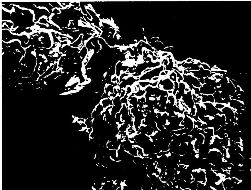
Figure 1.12. The surface microstructure of the reduced synthetic ilmenite (particle size \cong 70 \mu\text{m} ; sample coated with Au/pd); specimen tilt, 30^\circ ; magnification, 1050X; left bar length, 10 \mu\text{m} .
