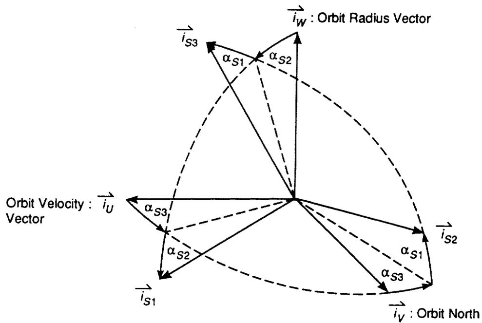
Figure 2. Satellite axes referenced to orbital coordinates.
