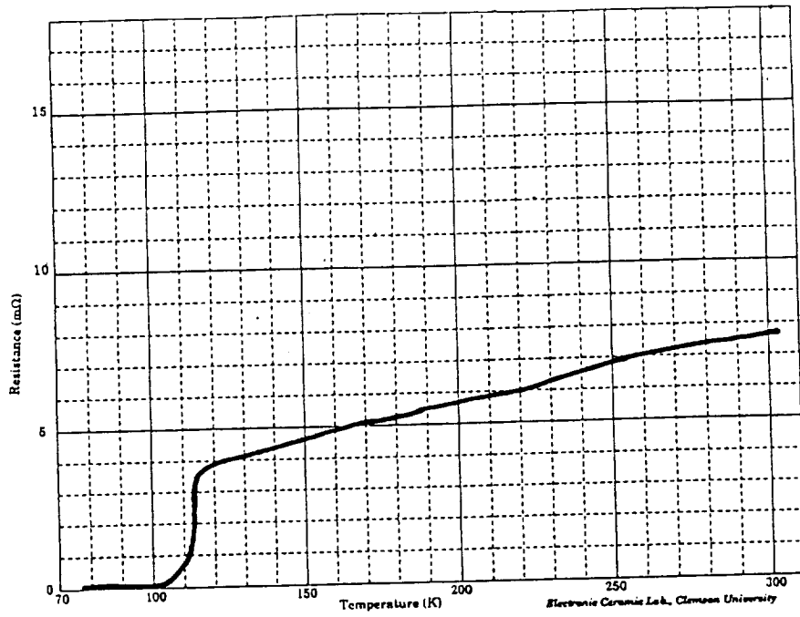
c) Pellet with a fast heating rate and slow cooling rate. The T_c was 101.4 K.
