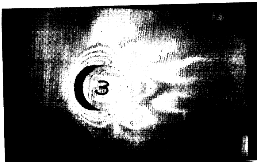
Figure 4.1d. Circular Cylinder, ISU Wind Tunnel, Height H = 8.6 cm, Diameter D = 13 cm, D/H = 1.5 , u_* = 0.73 m/s, U_h = 7.1 m/s, U_h D/\nu = 75400 , u_*^3/g\nu = 2570 , U_h t/D = 17200 , U_h^2/gD = 31.9 . This figure illustrates the moiré fringe pattern.
