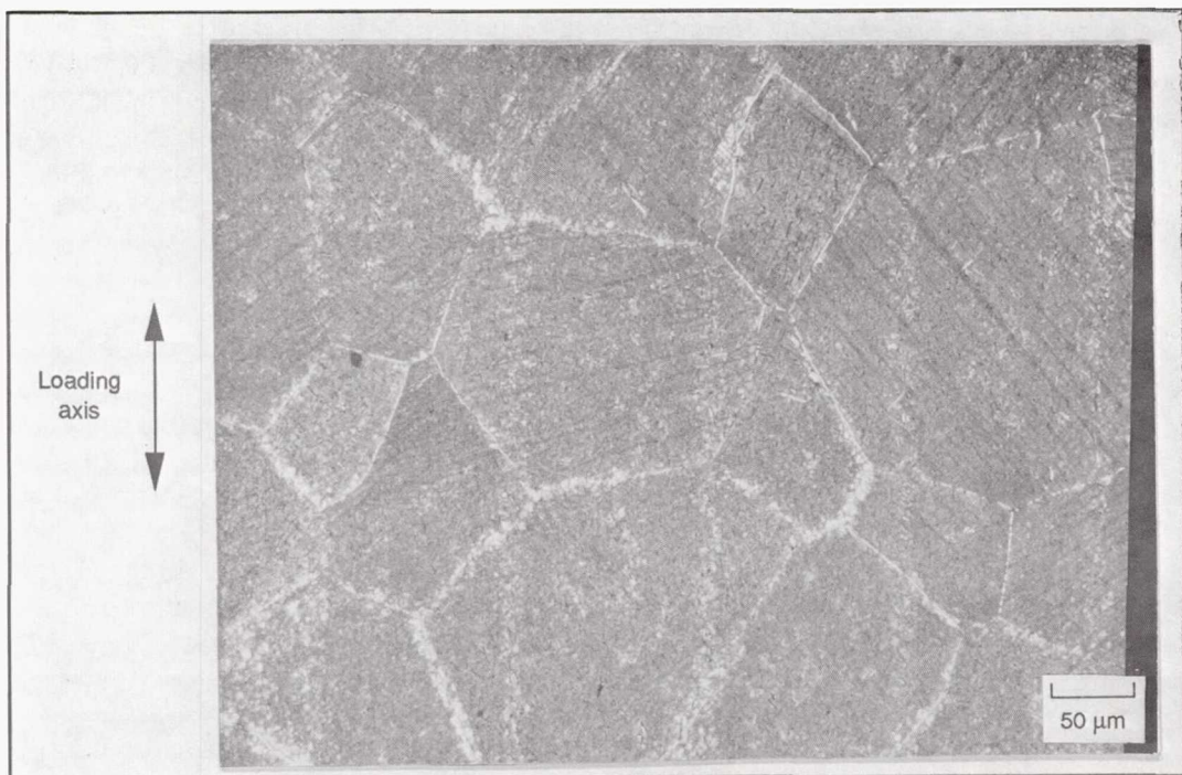
Figure 2.—Enlargement of the transition area "A" in figure 1 showing slip bands in some grains.
