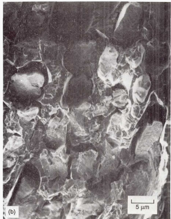
Figure 12. - Fracture behavior of a Ni-30Al alloy with a directional solidification rate of 0.5 cm/hr.
