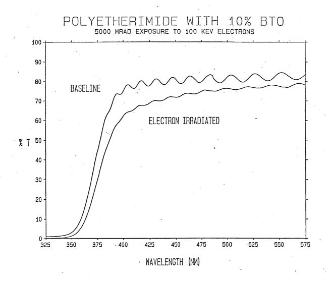
Figure 8. The uv/visible spectra of a polyetherimide film with 10% BTO before and after exposure to 100 keV electrons.
