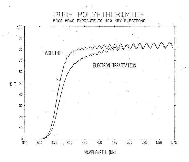
Figure 7. The uv/visible spectra of a pure polyetherimide film before and after exposure to 100 keV electrons.
