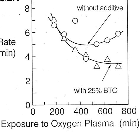
Figure 3. Erosion rates of films in atomic oxygen. A comparison of polyetherimide films pure and with 20% BTO.
