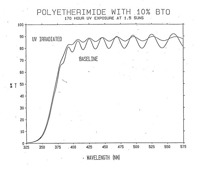
Figure 6. The uv/visible spectra of a polyetherimide film with 10% BTO before and after exposure to ultraviolet radiation.
