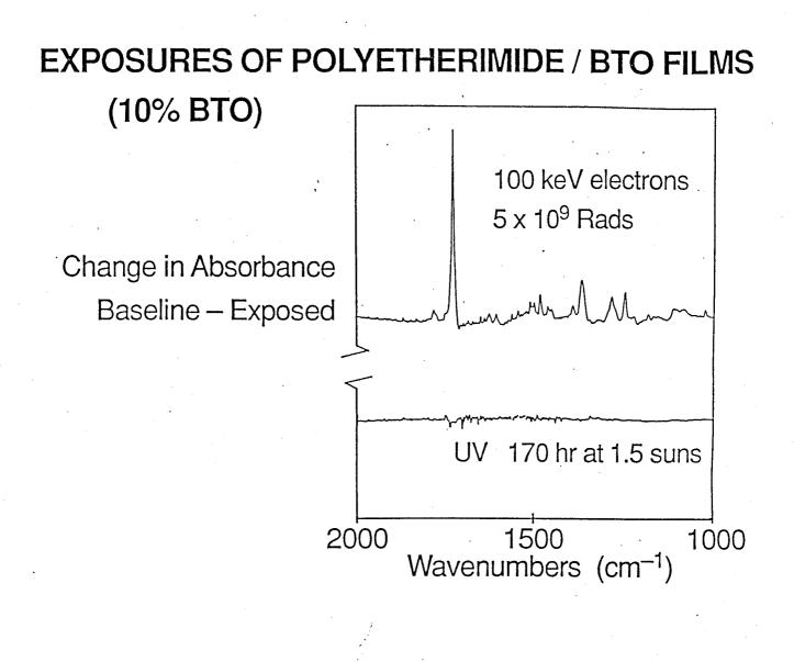
Figure 4. The difference in the infrared absorbance spectra of polyetherimide/10% BTO films taken before and after exposure to 100 keV electrons and ultraviolet radiation.
