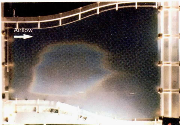
(a) Higher temperature liquid crystal, early in test run.
