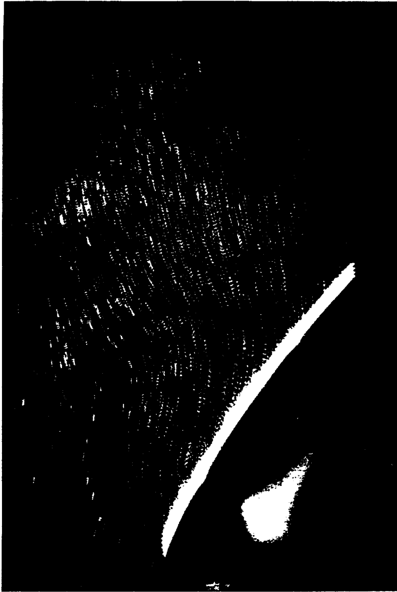
Figure 9b. Double-Exposed Photograph of Airfoil Impulsively Started from Rest; Biased Image
