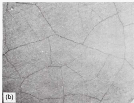
(a) No surface macrocracking for oxidized sample 2. (b) Surface macrocracking for oxidized sample 5.
