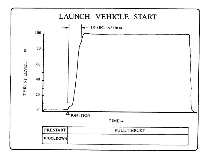
For a space application where gravitational losses are not as critical, a more efficient engine start sequence is possible.
