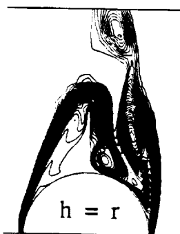
Figure 8. Passive flow control using a vertical fin, h = r , full Navier-Stokes solution.
