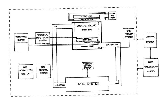
Figure 1. Block diagram of component subsystems and physical zones of the Crop Growth Research Chamber (CGRC).
