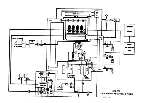
Figure 2. Functional design of the Crop Growth Research Chamber.
