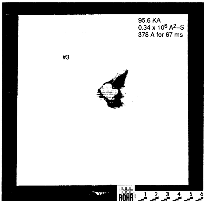
Figure 11.—Lightning strike damage on a painted bromine intercalated P-100 pitch-based carbon fiber/epoxy composite.
