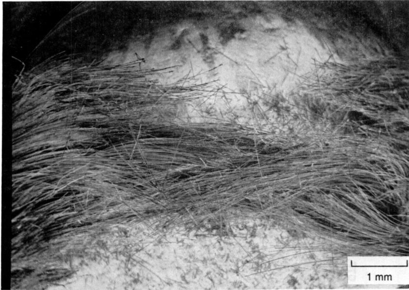
Figure 8.—Nextel 440 Hf fiber-pin specimens after testing at 900 °C. Virtually all of the fibers were broken during the test indicating low durability.
