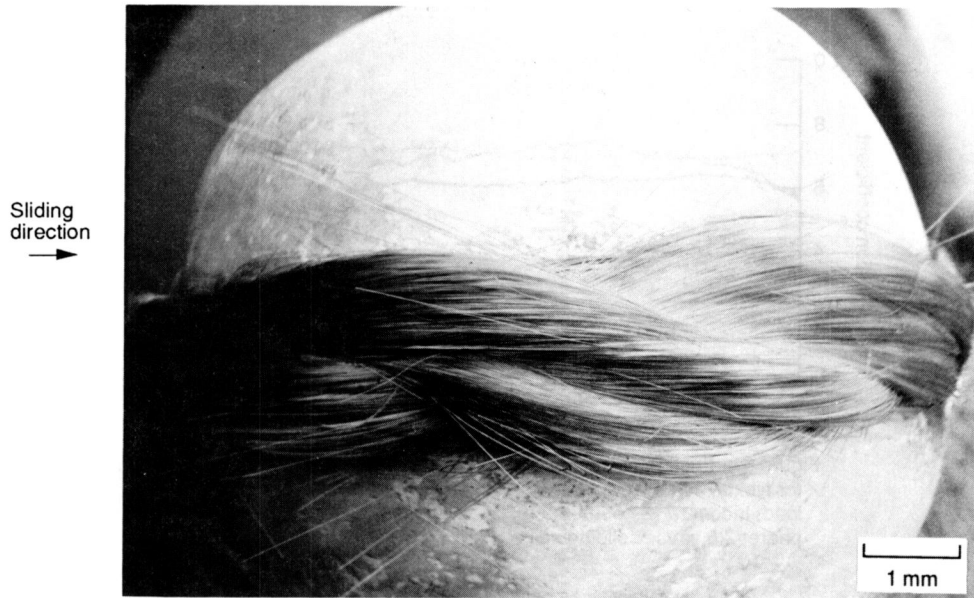
Figure 4.—SEM photomicrograph of fiber-pin specimen prior to testing. Sliding direction is from left to right.
