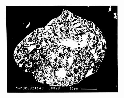
Fig. 1: Back-scattered electron photograph of a cross-section of a recovered fragment taken on the scanning electron microscope. The bright white region is the molybdenum metal and the dark gray region is the basaltic glass. This fragment was shocked to 6 GPa and shows intimate intermixing and reaction between the molybdenum and the basalt.
