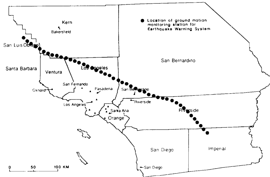
FIGURE 2. Schematic of sensor locations (10 km spacing) for an earthquake warning system to monitor the southernmost San Andreas Fault (from Holden et al. , 1989).
