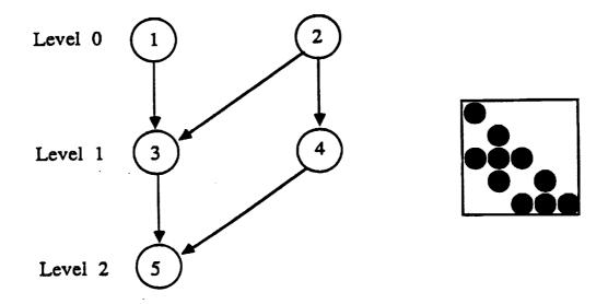
Figure 4: Illustration of the concept of Level.
