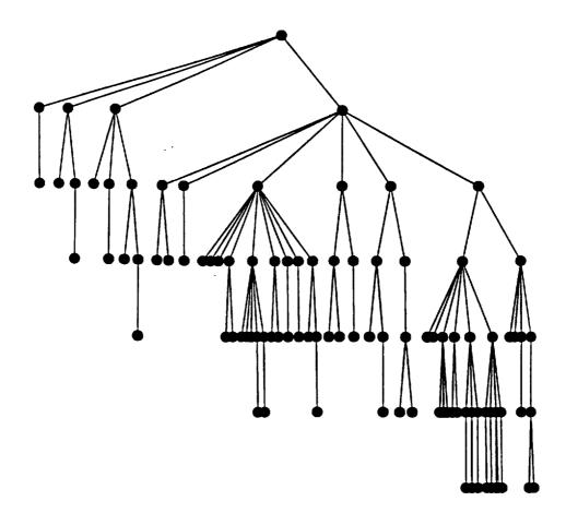
Figure 14: Clique tree for 118 node power system matrix with MLMD primary ordering, re-ordered and partitioned using RP1. This matrix has 99 maximal cliques and seven levels.
