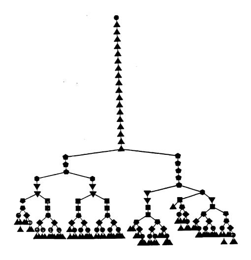
Figure 11: Elimination tree for finite difference grid matrix with MLMD primary ordering and partitioned using P1. The nine partitions are denoted by different shapes and shadings of the nodes (a tenth partition involving the last node only is trivial).
