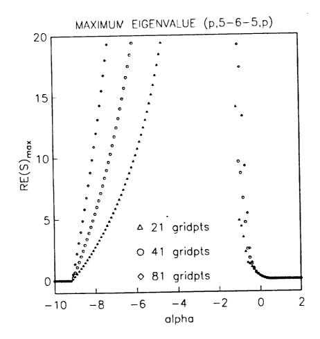
Fig-10 The maximum real part of the numerically determined eigenvalue spectrum, resulting from a sixth-order Pade inner scheme and a one-parameter family of third-order boundary schemes. The ordinant  $\alpha$  is the boundary parameter.
