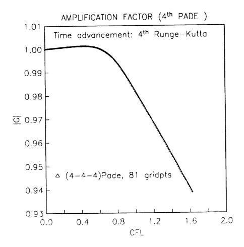
Fig-8 The maximum numerical amplification factor as a function of CFL, plotted for the uniformly fourth-order Pade scheme, with a fourth-order Runge-Kutta time advancement scheme.
