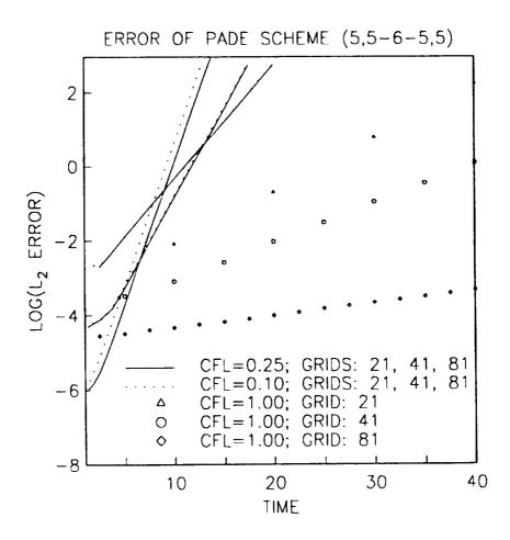
Fig-13 The  $L_2$  error as a function of time, resulting from the uniformly sixth-order Pade scheme with fifth-order boundary closure (5,5-6-5,5), for various CFL's and grid densities.
