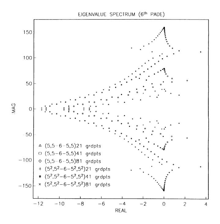
Fig-14 The numerically determined eigenvalue spectrum resulting from the sixth-order Pade inner scheme, closed with conventional fifth- or newly developed fifth-order boundary schemes, on various grids.
