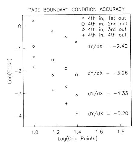
Fig-2 Comparative study of the effects of outflow boundary closure on the formal accuracy of the fourth-order compact inner scheme.
