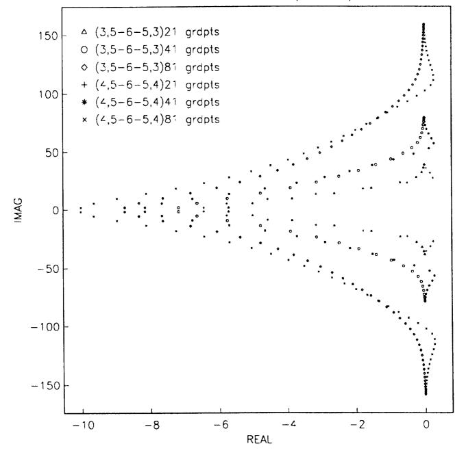
Fig-11 The numerically determined eigenvalue spectrum resulting from the sixth-order Pade inner scheme, closed with either third- or fourth-order boundary schemes, on various grids.
