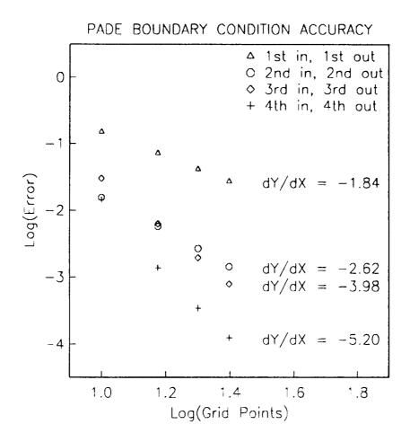
Fig-1 Comparative study of the effects of boundary closure on the formal accuracy of the fourth-order compact inner scheme.
