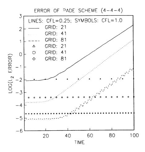
Fig-5 The  $L_2$  error as a function of time, resulting from the uniformly fourth-order Pade scheme (4-4-4), for various CFL's and grid densities.
