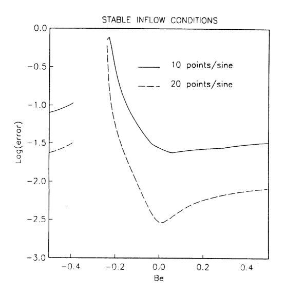
Fig-4 Numerical determination of the  $L_2$  error at a time level "T" resulting from a oneparameter family of closure formulas at the inflow boundary. The inner scheme is the fourth-order Pade scheme.
