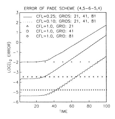
Fig-12 The  $L_2$  error as a function of time, resulting from the uniformly sixth-order Pade scheme with fourth-order boundary closure (4,5-6-5,4), for various CFL's and grid densities.
