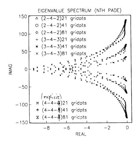
Fig-9 The numerically determined eigenvalue spectrum resulting from the fourth-order Pade inner scheme, closed with either second-, third- or newly developed fourth-order boundary schemes, on various grids.
