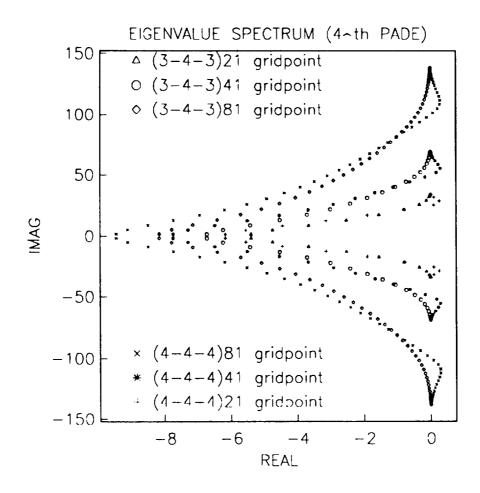
Fig-7 The numerically determined eigenvalue spectrum resulting from the fourth-order Pade inner scheme, closed with either third- or fourth-order boundary schemes.
