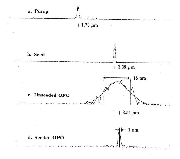
Fig. 1. Line Narrowing as a Result of Injection Seeding AgGaSe<sub>2</sub> Optical Parametric Oscillator. Observed linewidths of pump and seed beams are instrument limited. The output linewidth of the seeded OPO becomes narrower than the resolution limit.
