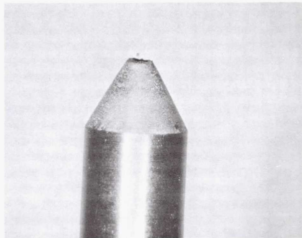
(b) Photograph of arcjet cathode after use with Nozzles A, B, and C. Represents 141 starts and approximately 28 hrs of operation using H_2 . Tip receded a total of 1.27 mm.
