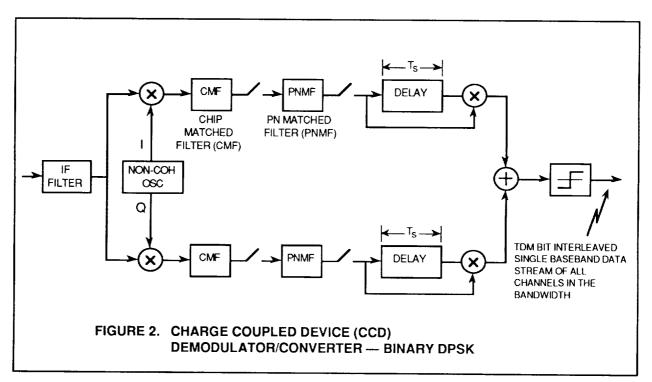
code phase with all other users producing minimum correlation. The sequence of correlations within the PNMF thus produce a sequence of despread samples corresponding to each user's data symbol in turn. These samples are then processed using conventional DBPSK methods to yield a single Time Division Multiplexed (TDM) baseband data stream consisting of all symbols from all users.
