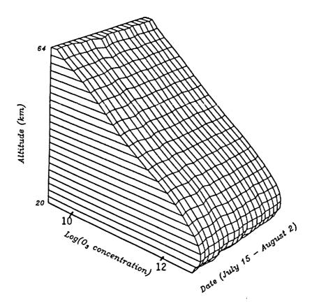
Nighttime ozone measurements during STOIC with the millimeter-wave spectrometer. Units of concentration are  $\mbox{cm}^{-3}.$
