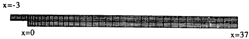
Fig. 11 Computational domain and grid distribution for backward-facing step flows (only every other grid lines are shown).
