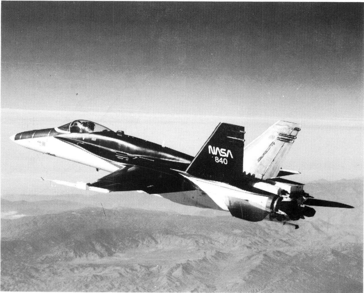
Figure 1. The F/A-18 high alpha research vehicle with the thrust vectoring control system installed.
