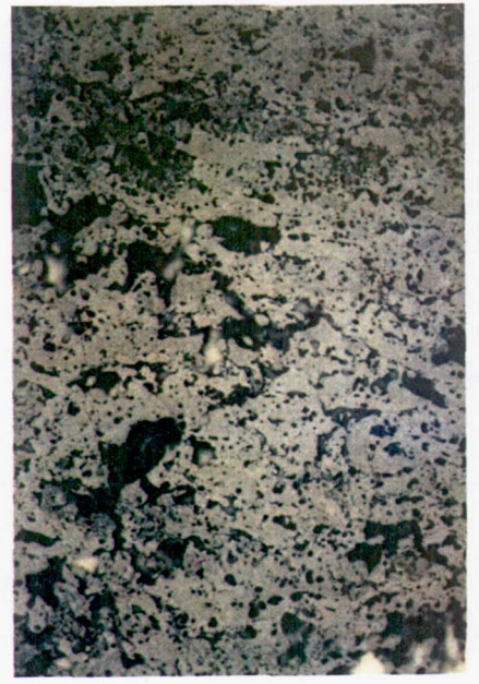
(c) Fluorescence. Epodye with blue excitation and yellow emission (green filter system).
