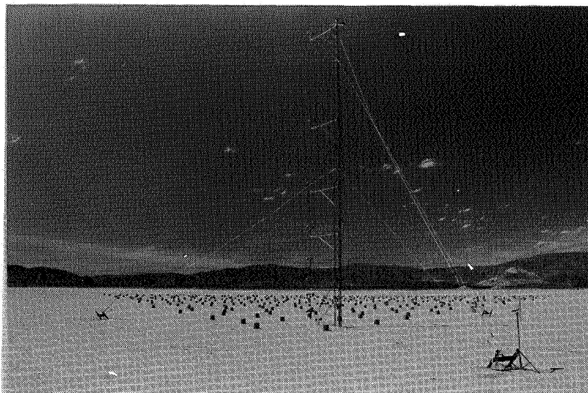
Figure 2. The full scale roughness element arrays on the eastern edge of Lucerne Dry Lake, California. (a) Array 1 looking into the prevailing wind direction (west). Upwind fetch = 89.6 m, roughness element spacing = 3.2 m. Mountains are 5-6 km distant.
