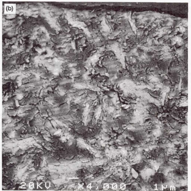
(a) Cross section of worn surface. (b) Cross section of the as-coated area of dry-film-lubricant.
