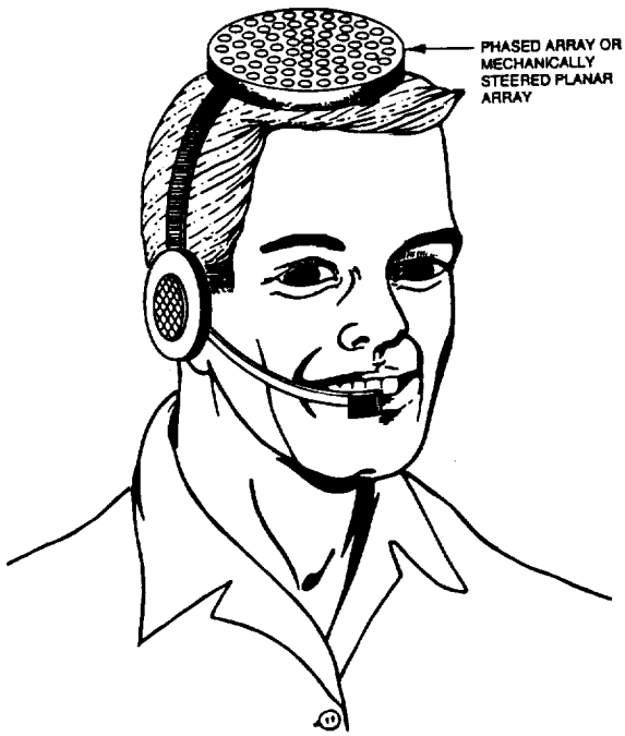
Figure 13. Head-mounted array antenna.
