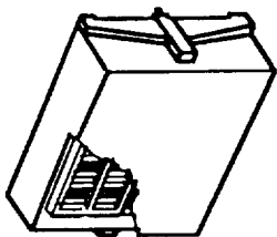
TRANSPORTER ENERGY STORAGE SUBSYSTEM
