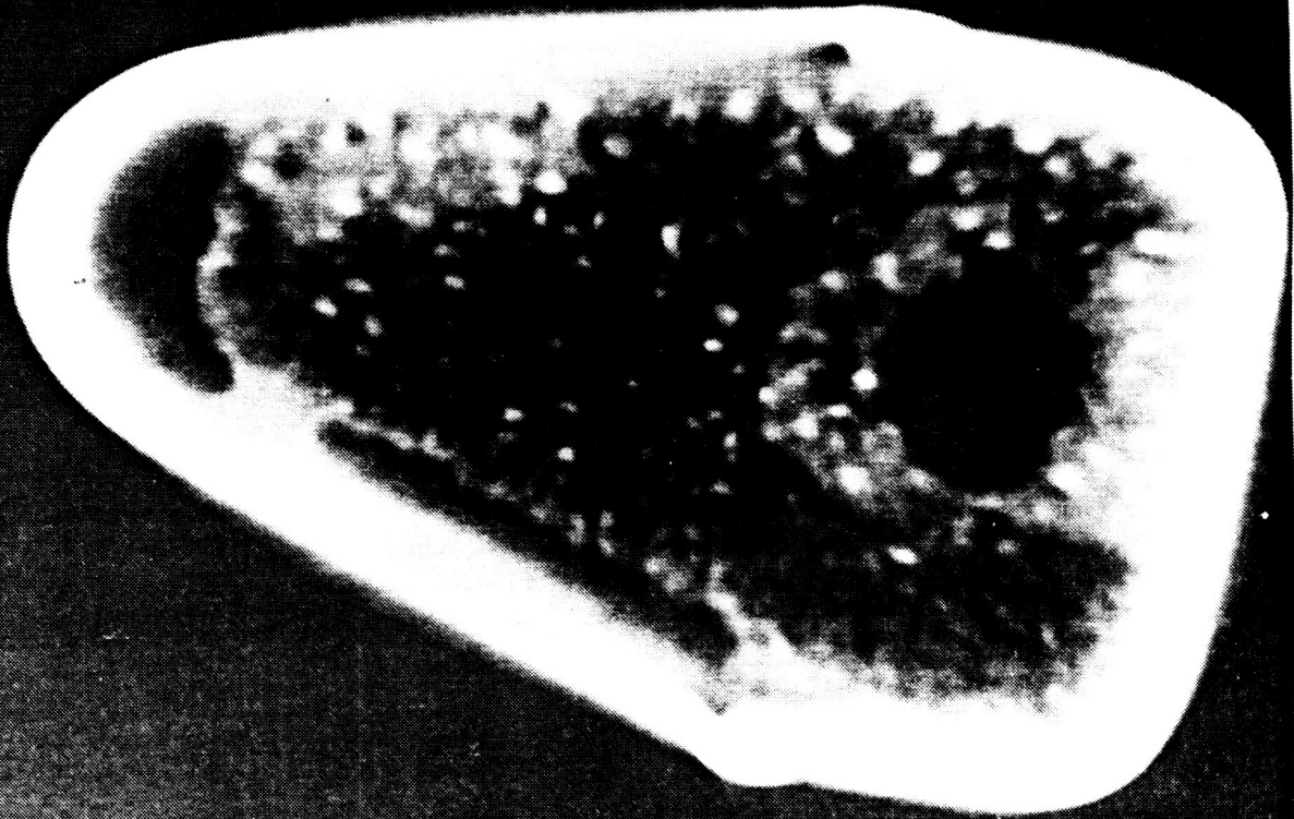
Figure 60 - CT IMAGE OF SECTION 3.0 INCHES FROM BOTTOM OF CANISTER
