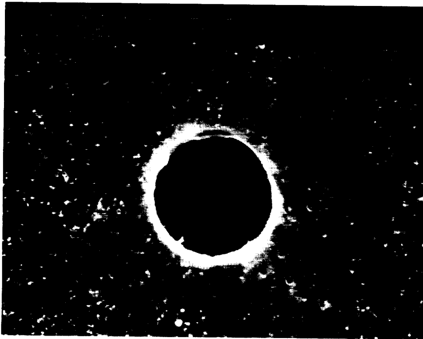
FIGURE 10. PERFORATION EVENTS IN IMPACT FILM
