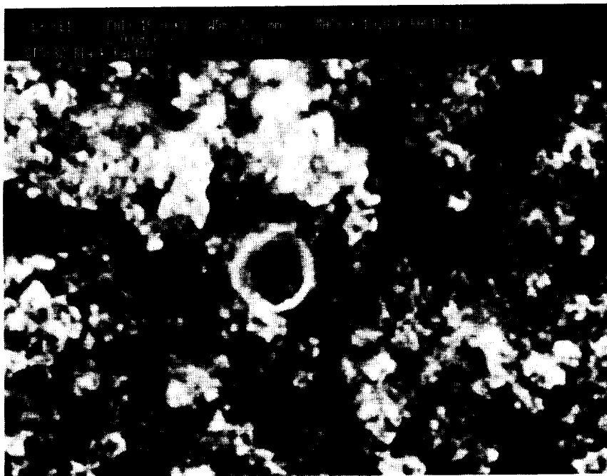
FIGURE 9. PERFORATION OF IMPACT FILM AND LDEF THERMAL BLANKET RESIDUE
